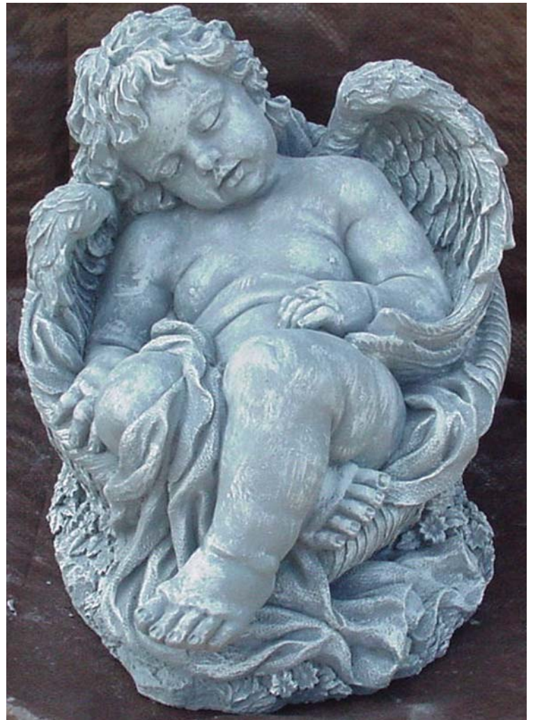
For 22 years Texas Traditional Molds have used latex rubber for the liner of their molds and fiberglass for the backing of the molds. This process allows for a detailed and durable finish product.
