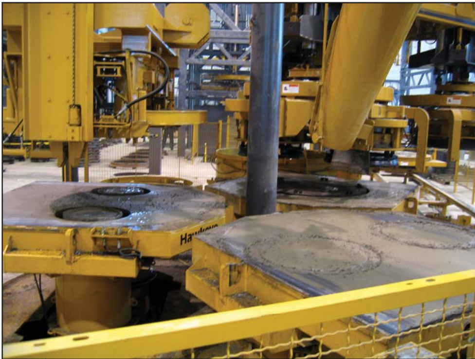
The PipePro Machine manufactures three different pipe sizes at-a-time on a rotary turntable.
