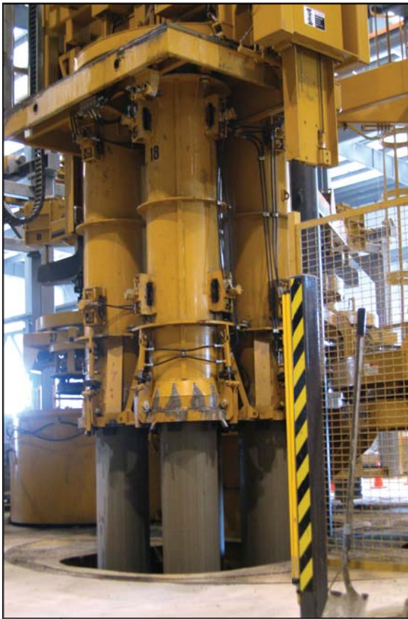
Quadform module is shown offbearing four pipe at-a-time from the PipePro Machine. All pipe sizes up to 18" diameter are produced with Quadform modules for maximum output.
