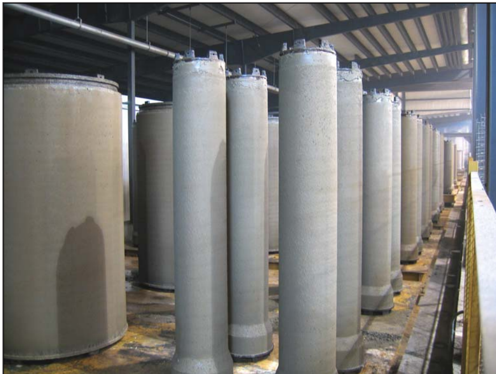
Pipes are transported to curing chambers with a circulating moving floor system that permits continuous or any length production shift.
