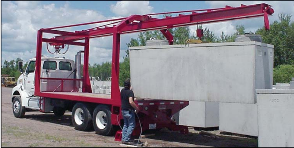
Product is unloaded or loaded directly behind the truck. Simple action: up, down, in, out, left and right.
