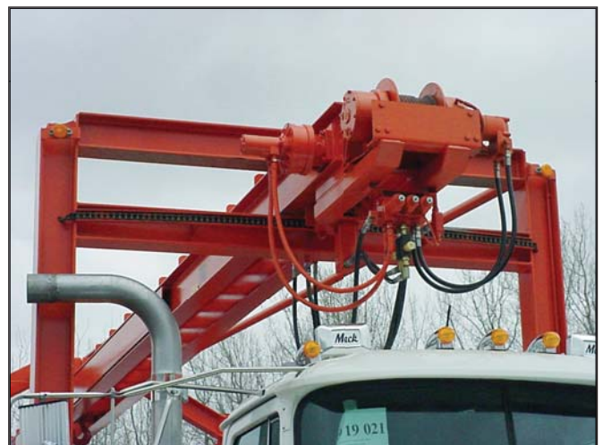
fewer moving parts on a rail boom compared to a knuckle boom, maintenance is minimized.
